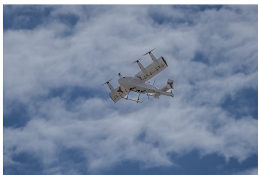
FIGURE 1 Fully electric aerial drone taking off for kidney graft transport during a preclinical experiment in France. The propulsion system consists of four rotors positioned vertically during takeoff and landing, which tilt horizontally during cruising flight. Image courtesy of Dufour Aerospace (Dübendorf, Switzerland).
