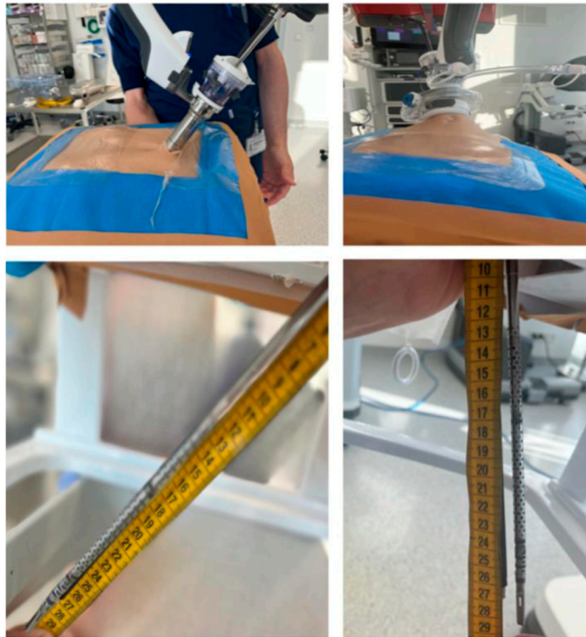
FIGURE 2 | Ex vivo exploration performed using a Dietz' silicone abdominal wall model to determine the ROM and reach of the instruments using the Da Vinci SP robotic system either with a metal cannula or with the SP small access port. (courtesy of Prof Ulrich Dietz from Olten, Switzerland).
