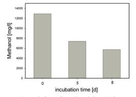
Figure 5. Degradation of methanol by *Trichosporon* sp. high-density culture  $(2.3 \times 10^7 \text{ cells/ml})$ .
