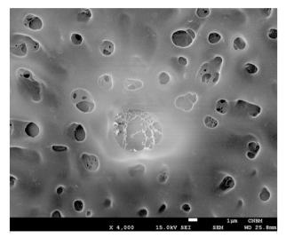
Figure 8. CRYO-SEM pictures of pNiPAM thermo-responsive nanogel; Close-up of the porous surface
