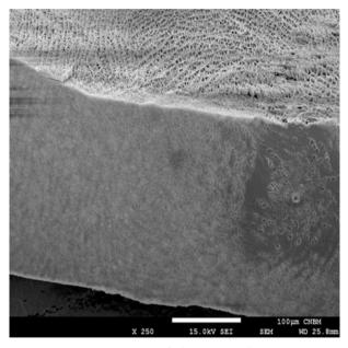
Figure 7. CRYO-SEM pictures of td-3 pNiPAM thermo-responsive nanogel showing the surface and the 'interior'.
