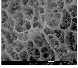
Figure 9. CRYO-SEM pictures of pNiPAM thermo-responsive nanogel; Close-up of the porous interior.
