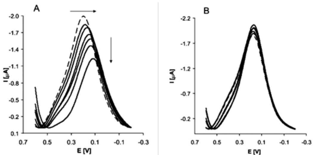
**Figure 3.** Typical Osteryoung square wave voltammograms obtained for electrodes modified with HS-ssDNA and 6-mercaptohexan-1-ol upon hybridization.
