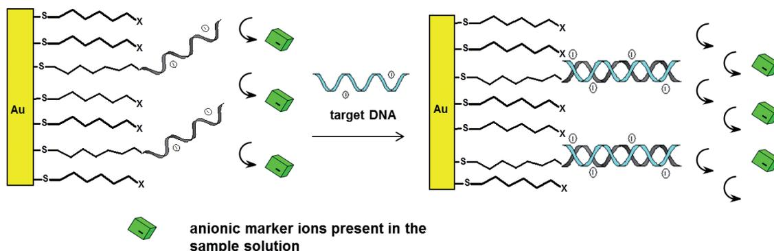
Figure 2. A scheme of the working principle of the ion-channel mimetic genosensor.
