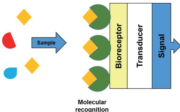
Figure 1. Schematic structure of a biosensor.
