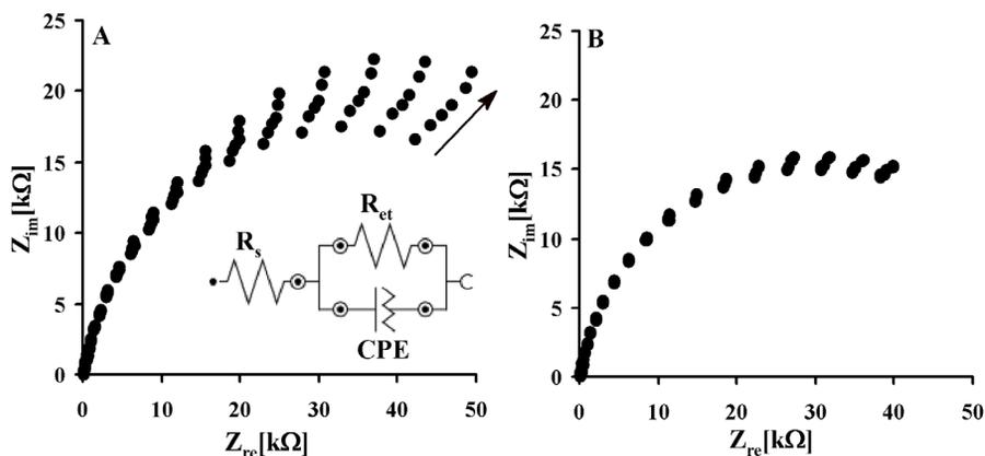
**Figure 8.** Electrochemical impedance spectra of BSA/long His<sub>6</sub>-H5 HA/anti-His/protein A modified electrode (a) in buffer solution and after treatment with diluted hen serum with PBS buffer: (b)  $7 \times 10^7$ , (c)  $7 \times 10^6$ , (d)  $7 \times 10^5$ , (e)  $7 \times 10^4$ , (f)  $7 \times 10^3$ .
