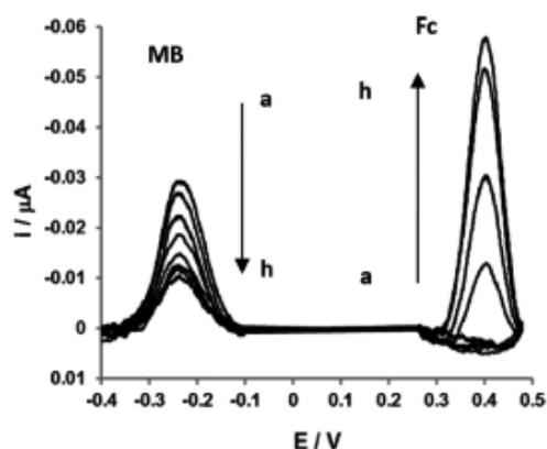
Figure 5. Representative Osteryoung square wave voltammograms obtained for electrodes modified with (a) SH-ssDNA-Fc probe and SH-ssDNA-MB probe and after hybridization with (b) 8 nM, (c) 10 nM, (d) 20, (e) 40, (f) 60, (g) 80 and (h) 100 nM oligonucleotides sequences complementary to SH-ssDNA-Fc and SH-ssDNA-MB.
