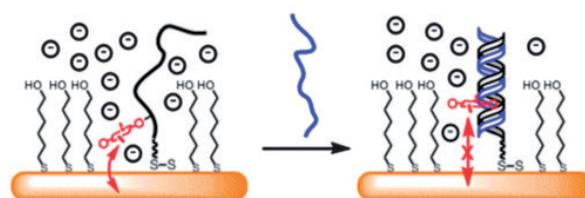
Figure 7. Schematic illustration of the signal generation mechanism of the Co-porphyrin-DNA genosensor.
