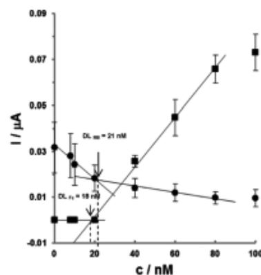
Figure 6. Change of peak current recorded for electrodes modified with (■) SH-ssDNA-Fc probe and (●) SH-ssDNA-MB probe vs. concentration of particular complementary sequences: from 8 to 100 nM ( $n=4$ ).
