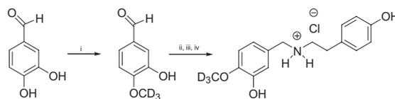
**Figure 2.** Steps of 4'-O-methyl-d<sub>3</sub>-norbelladine synthesis. Reagents and conditions: (i) CD<sub>3</sub>I, K<sub>2</sub>CO<sub>3</sub>; (ii) tyramine, molecular sieves; (iii) NaBH<sub>4</sub>; (iv) HCl.
