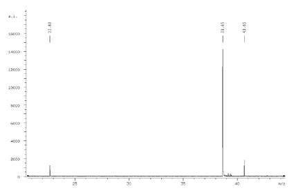
Figure 2. DIOS mass spectrum of empty spot irradiated with laser.
