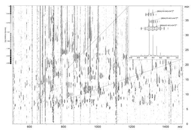
Figure 2. A contour plot of the result from an LC-FTICR MS experiment of a tryptic digest of bovine serum albumin.
