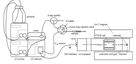
Figure 1. The micro-capillary liquid chromatography FTICR mass spectrometric experimental set-up.
