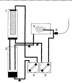
**Fig.1** Depiction of perfusion system. (1 oxygenator, 2 reservoir, 3 perfusion chamber, 4 oxygenation pump, 5 perfusion pump, 6 pressure monitoring)
