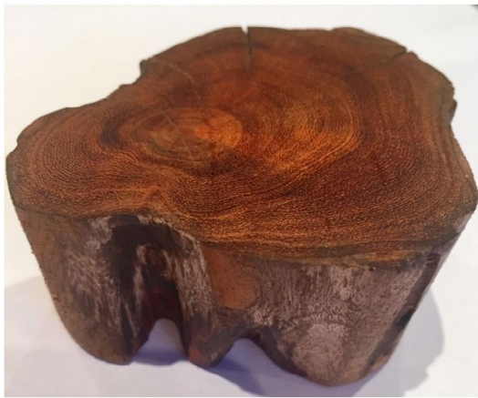
Figure 2. Photograph of a cross section of Haematoxylon campechianum logwood showing the rich vibrant colour of the wood used to extract haematin.
